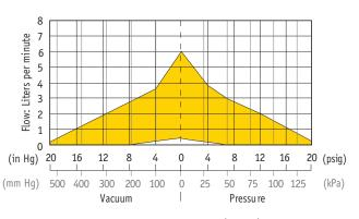
The above performance graph illustrates the overall performance of the TTC handling air at 800 feet (244 m) above sea level at 75° F (24°). Performance will vary depending on barometric pressure and media temperature. Consult factory with your specific requirements.
